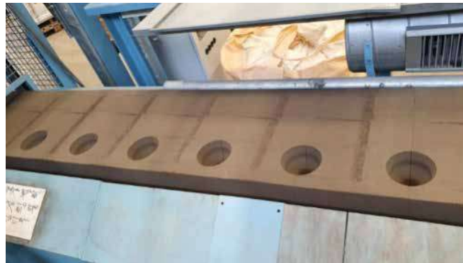
Figure 10 : Mould string ready for pouring.
