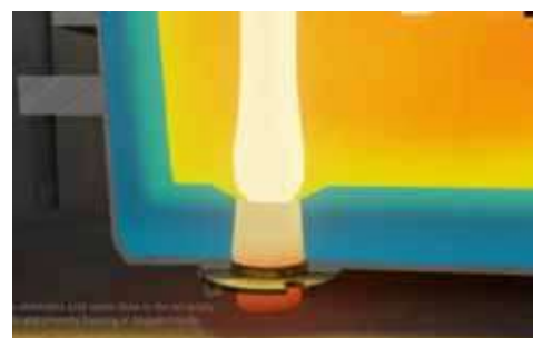
Fig4b: Metal temperature homogenization by ROTOCLENE - Rotary Treatment Process
