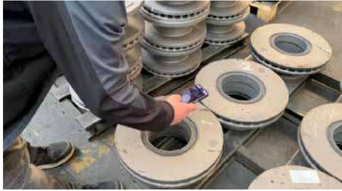
Figure 13: CDOT code reading on transferred CDOT code
