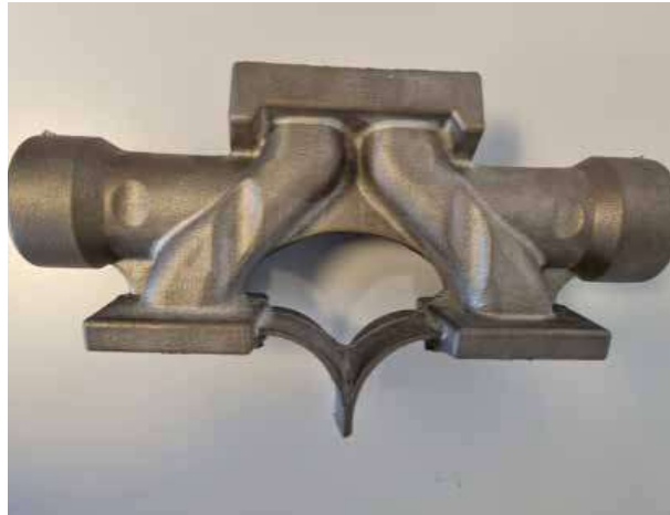
Figure 1 : A steel manifold produced in green sand.
