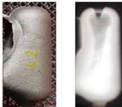
Figure 15 : X-ray of container corner casting feeder neck.
