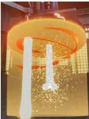
Fig 3a: Very fine Ar bubbles helically dispersed
