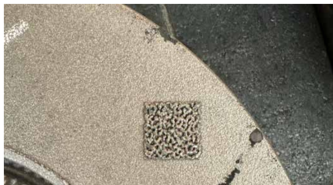
Figure 12: %100 readable CDOT code marked on sand mold, transferred to part during ore pouring
