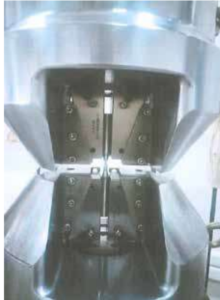
Figure 4: Test Configuration and Fatigue Limit Test Specimen [1]
