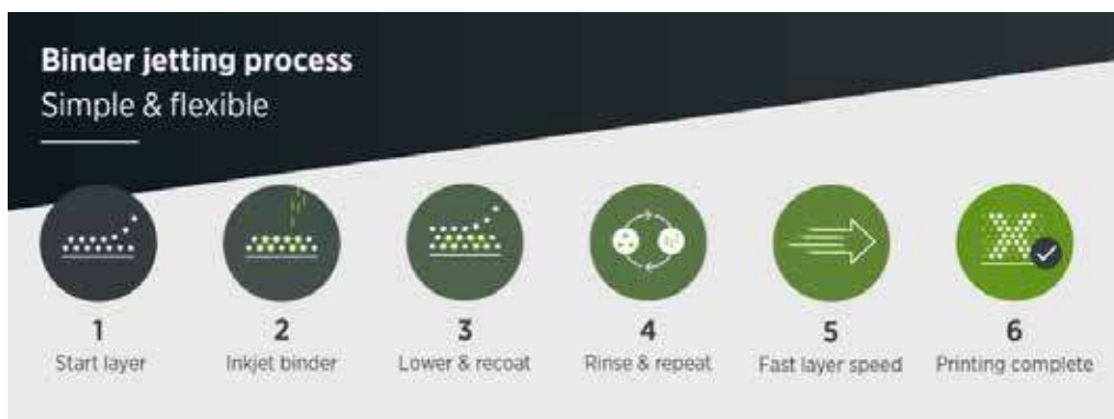
Figure 1: Binder jetting process
