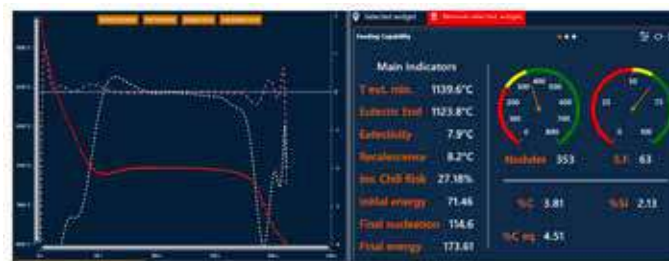
Figure 8: Cooling curve of thermal analysis showing the main features of the metal poured.
