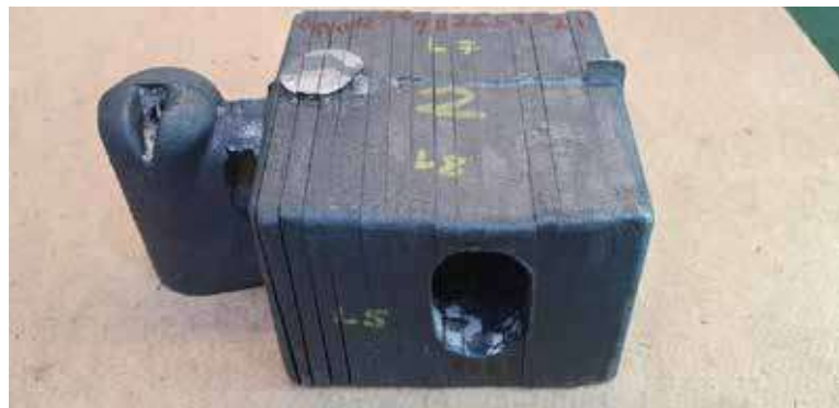
Figure 11 : Casting sliced for inspection.
