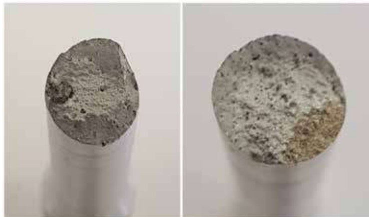
Figure 9: Fracture Surfaces of Specimen 3 and Specimen 6
