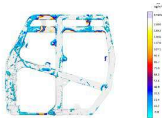
Figure 9: Air results of the part with air pockets obtained through simulation
