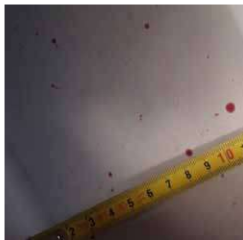
Fig 14b: Defects on the diameter are still present and needs to be further machined
