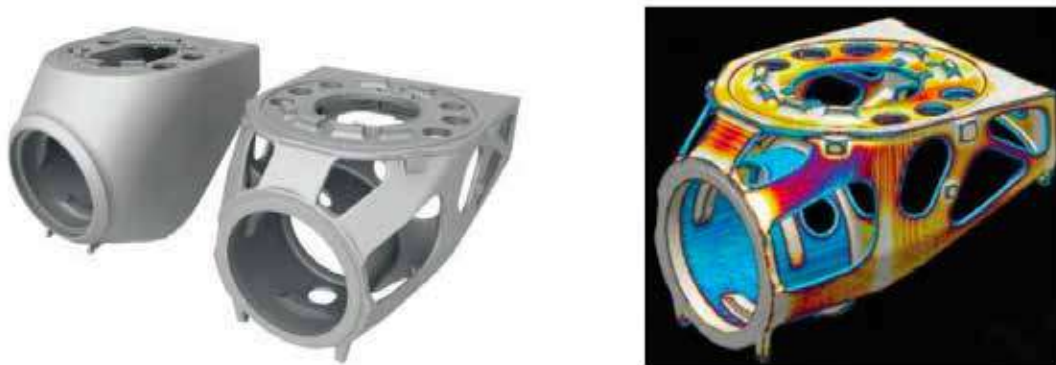
Figure 1: High tonnage casting part which design is changed with the topology method
