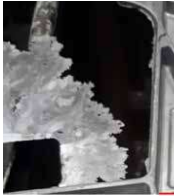
Figure 6: Flash formation due to exceeding mold closing force.
