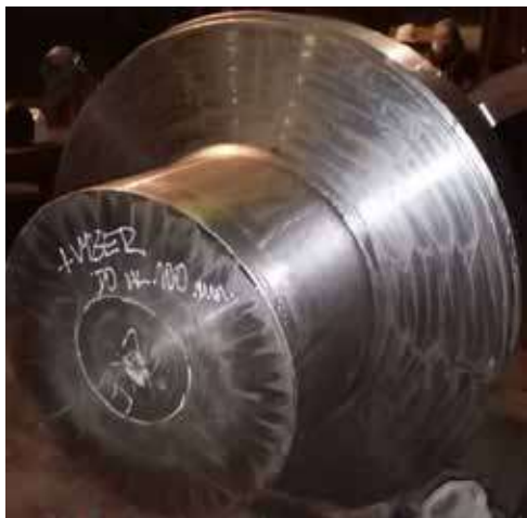
Fig 13a: Porosity in bottom hub
