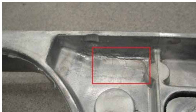
Figure 4: Effect of cracks on mold surface.
