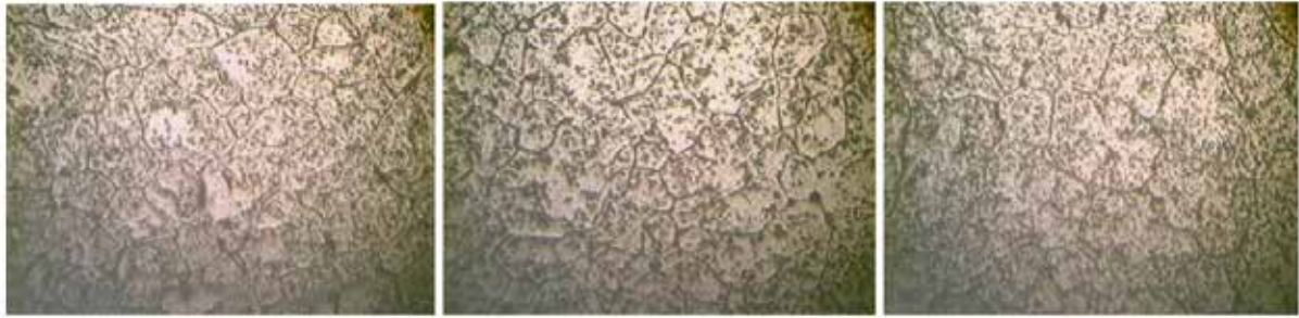
Figure 3: Microstructure of the Specimen 4,5,6(without vibration) in Optical Microscope at 400x Magnification
