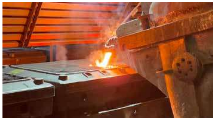
Figure 11: CDOT code transfer from sand mold to brake disc during pouring ore stage
