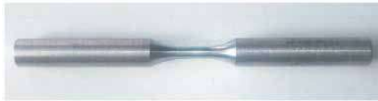
Figure 3: Fatigue Limit Test Specimen [1]
